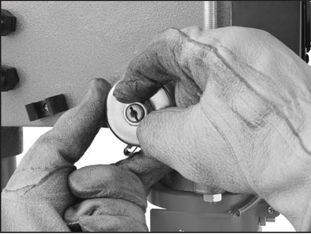
Figure 48. Example of loosening cover and jam nut.
