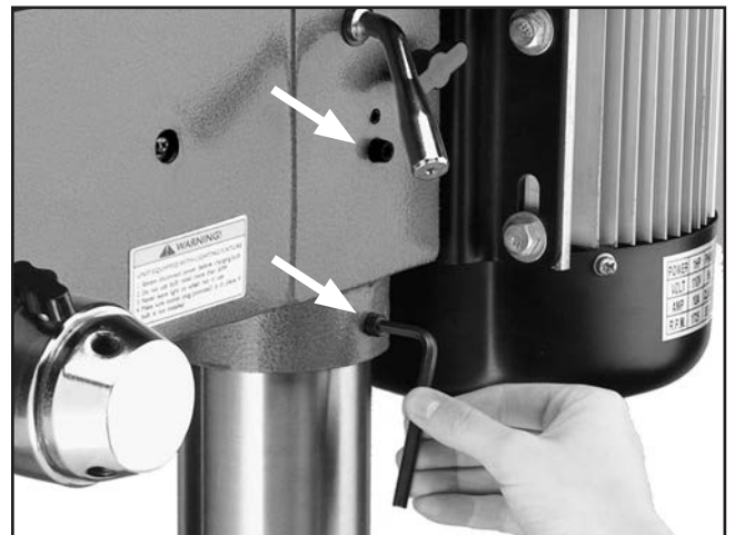
Figure 13. Securing headstock to column.
