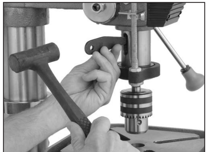
Figure 33. Using drift key to remove arbor.
