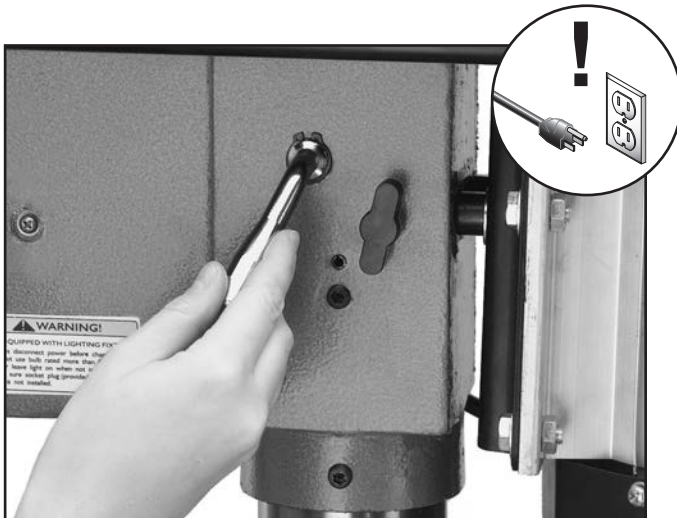
Figure 27. Using the belt tension lever.
