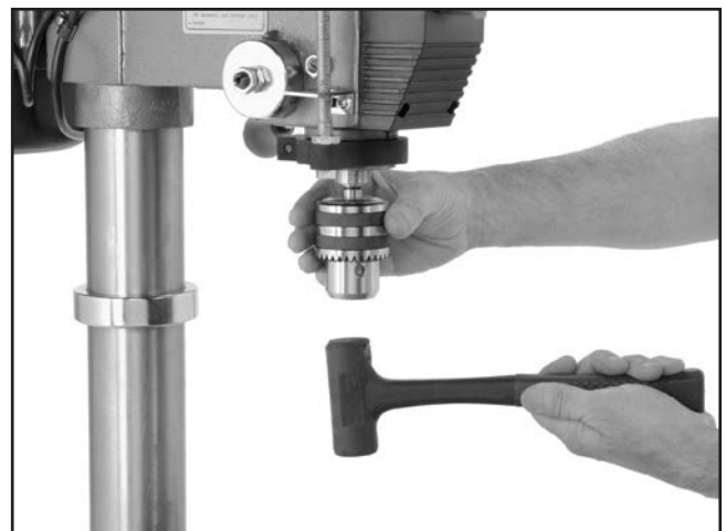
Figure 16. Seating arbor and chuck into spindle.
